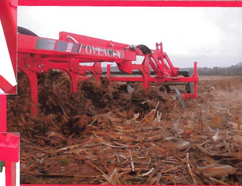
Leafspring auto reset protection. Decreasing trip pressure which protects the key structure of the Versatill. 100% maintenance-free Beams made of wear resistant, high elasticity steel
