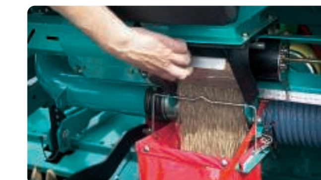
Time savings : the parts of the ADS system are centralised for an "express" calibration test and total emptying.
