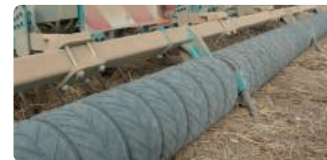
Soil firming: due to its integral Farmflex® roller (360 mm diameter), the Kronos saves you most of the time needed for post-drilling rolling! The angle-adjustable following harrow is also part of the standard equipment.
