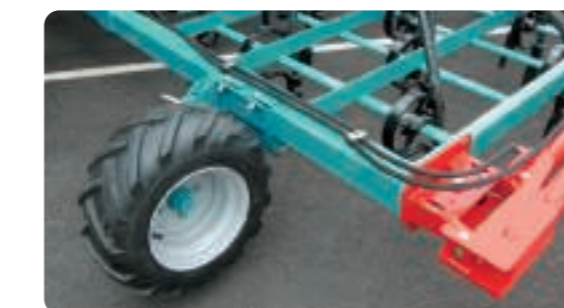
Front depth control wheels: recommended to deal with uneven seed beds at high speed.
