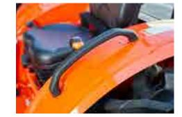
Armrest type handle grip on the fender will reduce the fatigue especially for the long time driver.
