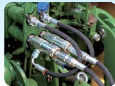
Hydraulic control with pilot controlled check valves(1) 2 DA
