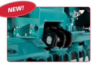
Reinforced solid couplerhead, allowing the incorporation of a seed drill with high hoppercapacity, due to the use of specialsteels and "top-of-the-range" screw fittings ...
